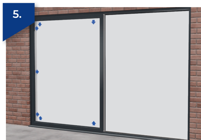
Remove fixed sash screws in glazing area.
